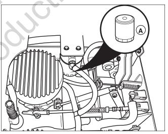
Figure 17. Change Hydraulic Oil Filter A. Hydraulic Oil Filter
